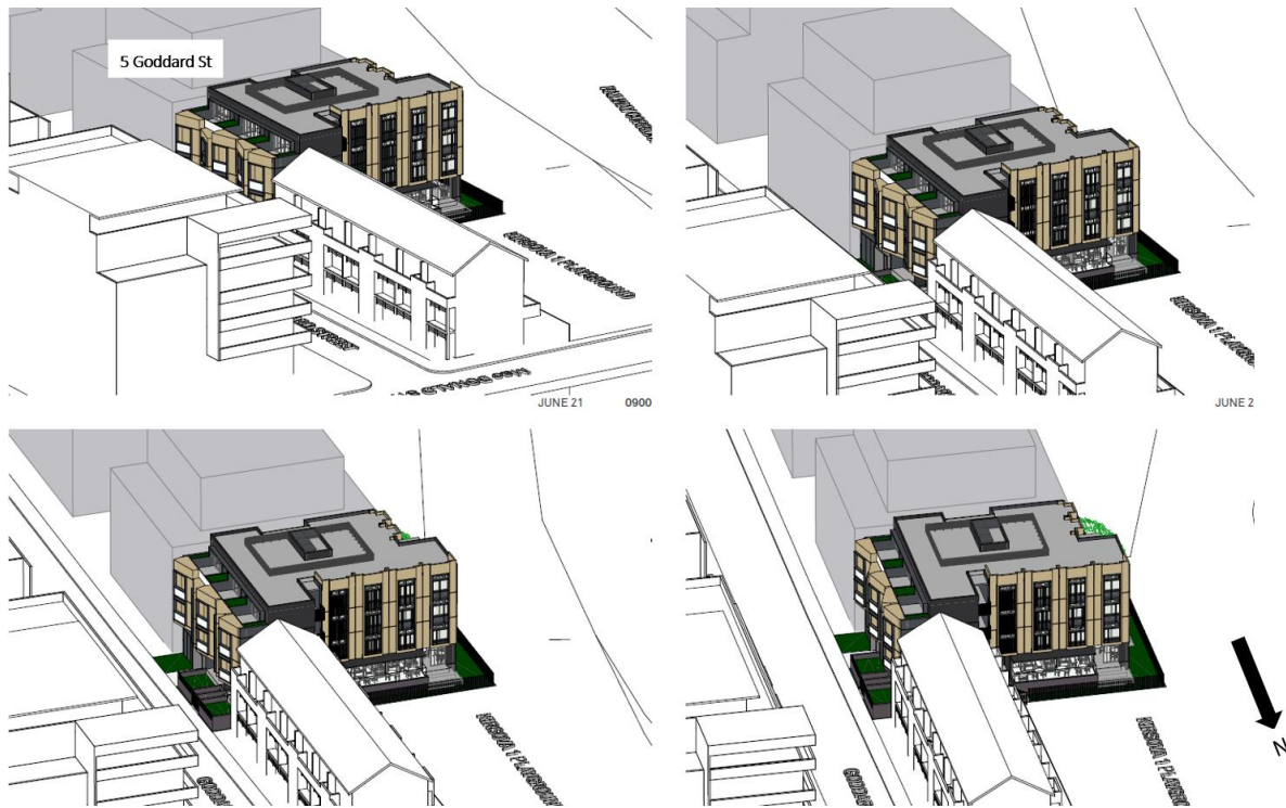
Figure 26: 'View from the sun' shadow diagrams show that future residential development within 5 Goddard Street will receive solar access to the eastern elevation prior to 11.00am on 21 June.
