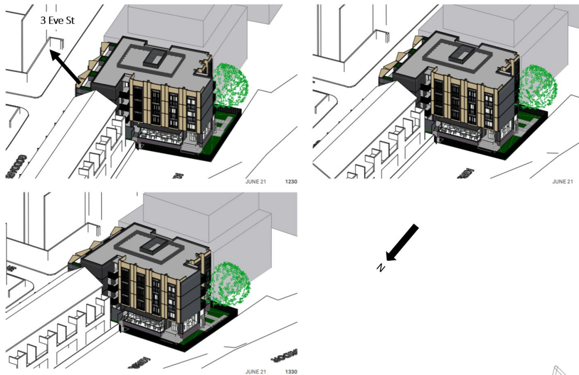
Figure 25: solar diagrams show that apartments within 3 Eve Street receive solar access between 12.00 midday and 2.00pm on 21 June.
